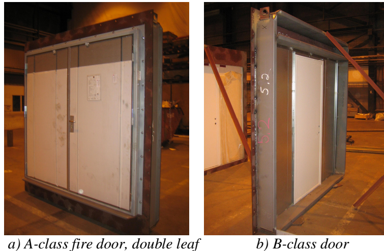
Fig. 5 a & b: Some examples of test specimens (doors & other structures to be tested) attached to the test frames, specially manufactured by STX, waiting for transportation to Gdansk, Poland, to be tested at CTO in WP2/Task 2.1. (Photos by STX)
