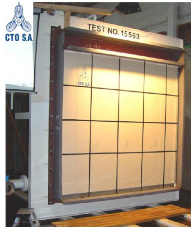
Figure 3 Test stand with a test specimen (in a frame) attached for the test in WP2/Task 2.1. In this case the test specimen is: cabin wall panel. (Photo: Deliverable D2.1b)
