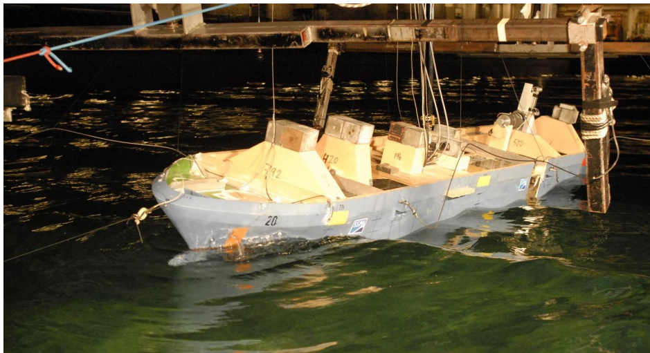
Figure 17 The 1:40 model of M/S Estonia in waves with the large opening in the aft (on the right side of this photo) representing constant parameter in all the tests (in WP4/Task 4.1)
