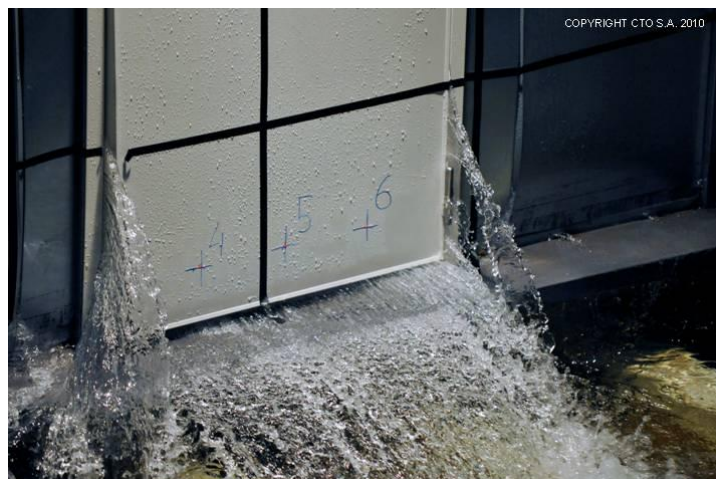
c) Close-up of the bottom part of a door in a test (Door deflection at points 4, 5 and 6 were measured with laser equipment)
