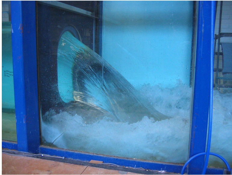
Figure 7 Flooding through a full-sized manhole in a flume tank tested in WP2/Task 2.3(Photo: Aalto University)
