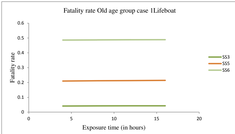
Figure 18: Fatality rate for the old age group in LB for HF+HW obstacles case 1
