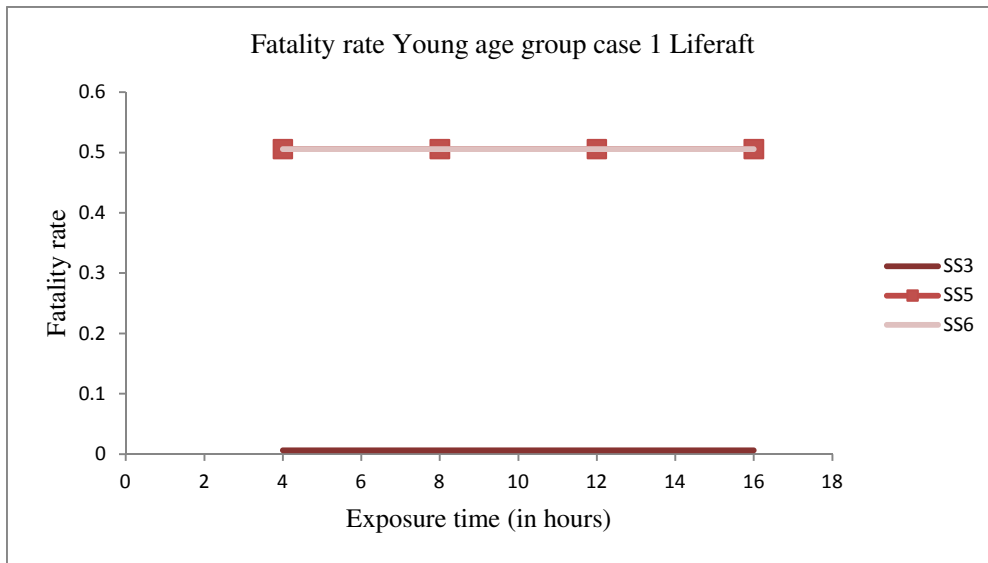
Figure 25: Fatality rate for the young age group in LR for HF+HW obstacles case 1
