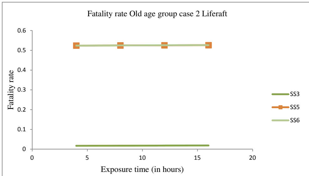
Figure 35: Fatality rate for the old age group in LR for HF+HW obstacles case 2
