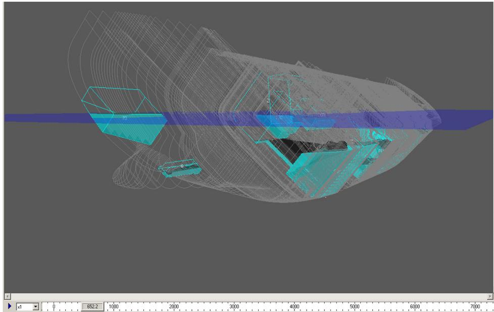
Figure 18 MV Rocknes, numerical reconstruction when heeling to 42 degrees during capsizing process. The vessel capsizes in 2 minutes. Visible in a light blue colour are the intact ship free surface tank loads as well as compartments flooded due to damage, Jasionowski et al 2005.
