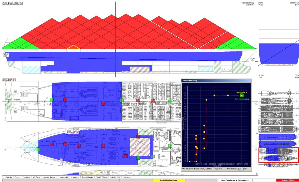
Figure 29 Flooding extent for damage case  $j=702$ , DS/S6.2.0, (diamond/triangle in yellow frame), with corresponding GZ curve logged at 19:00:30, ship vulnerability  $F_T(3hr|4m) = 68.24\%$ . Note  $H_s=4m$  and many WTD opened. Very likely state of the vessel on the night of the ship loss in September 1994.
