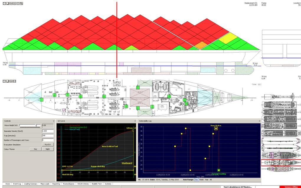
Figure 25 Screenshot of the colour-coded values of  $F_{T|*}(3hrs|H_s = 4m, j)$  for each of the flooding cases, ship vulnerability  $F_T(3hr|4m) = 37.18\%$  (purple window), logged down at 15:41:09 hours (example time marked by the yellow square at 15hrs 41minutes 09seconds). The green coloured “diamonds” indicate  $F_{T|*} = 0\%$ , and red  $F_{T|*} = 100\%$ . GZ curve and draught marks shown for the ship in intact condition. Sea state  $H_s$  manual input shown in the left lower corner.
