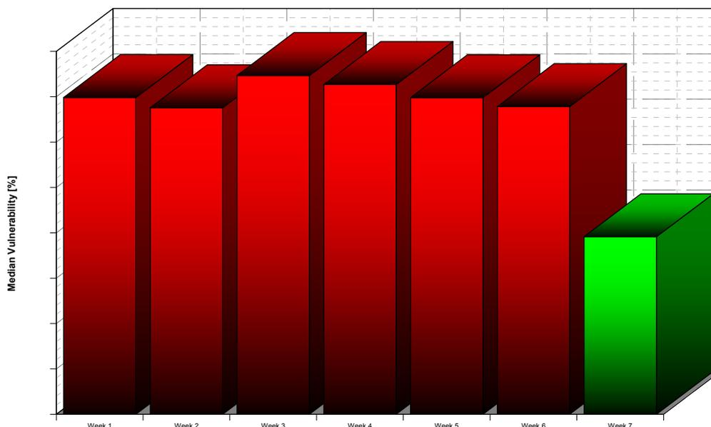
Figure 33 Median of vulnerability logged on a demonstration ship. The actual vulnerability values are undisclosed. The impact of the awareness of the crew on the day-to-day management of watertight integrity, and hence crew and ship preparedness, can be seen in the Week 7, when explanations and training on use of VLog had been given.
