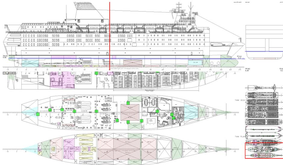
Figure 23 Ergonomic communication interface, model of MV Estonia, screenshot of watertight doors (WTD) closure status, green indicates “closed”, red “opened”.
