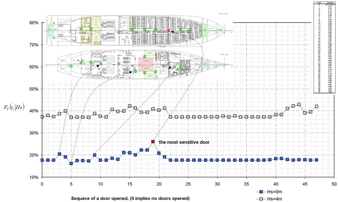
Figure 31 Impact of single doors opening on overall ship vulnerability.
