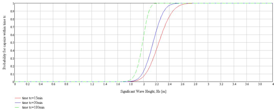
Figure 21 Probability for capsizing within time  $t_c$ . Case No 36 with all doors closed. Effect of significant wave height.
