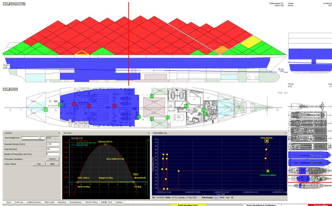
Figure 28 Flooding extent for damage case  $j=702$ , DS/S6.2.0, (diamond/triangle in yellow frame), with corresponding GZ curve logged at 16:15:28, ship vulnerability  $F_T(3hr|4m) = 44.93\%$ . Note  $H_s=4m$ .
