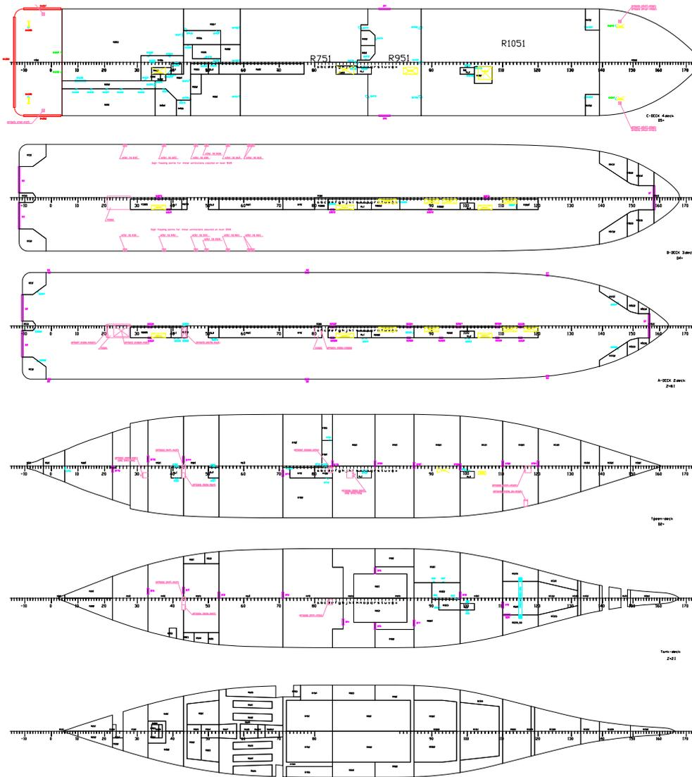
Figure 19 The GA of MV Estonia assumed for numerical modelling.
