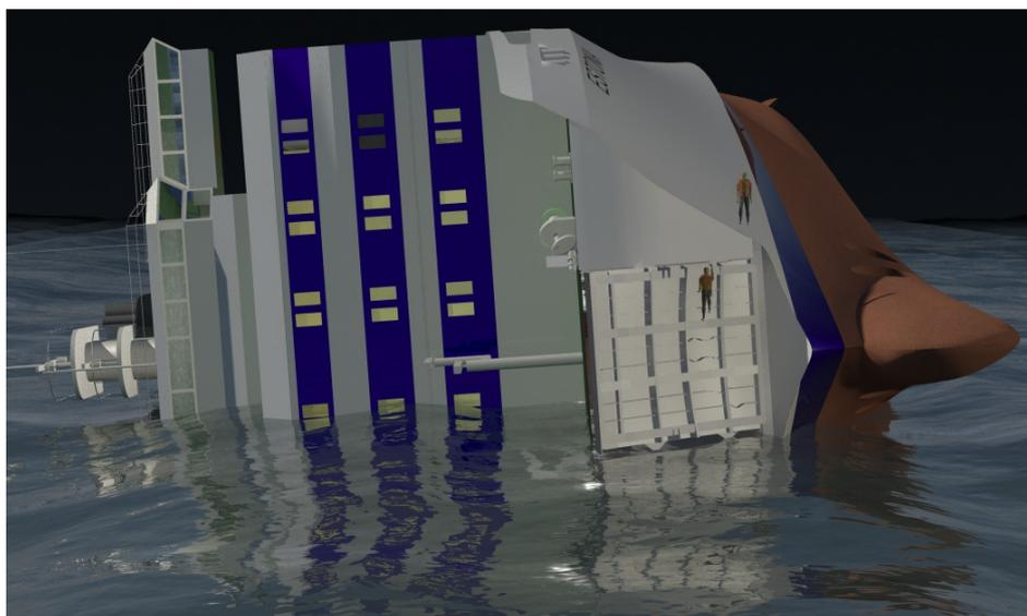
Figure 15 MV Estonia, Jasionowski et al 2008. At some instant two survivors managed to climb down the closed ramp, using its stiffening arrangement and abandon the ship. Heel angle 93deg.
