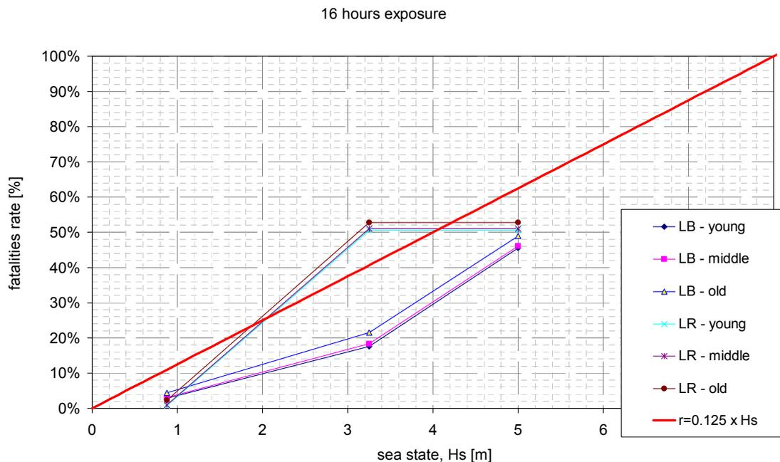
Figure 2 Rate of fatalities,  $E(N)/N_{\max}$ , as a function of sea state, age and type of LSA. Simplified criterion given by ( 7 ).
