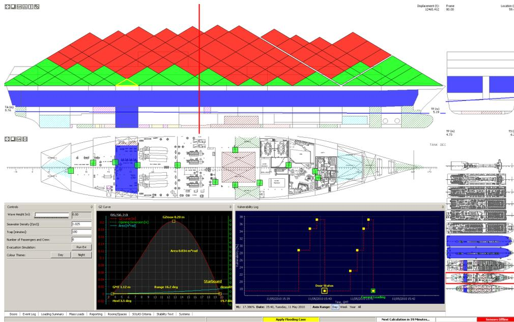
Figure 26 Flooding extent for damage case  $j=702$ , DS/S6.2.0, (diamond/triangle in yellow frame), with corresponding GZ curve logged at 15:40:06, see Figure 24. Ship vulnerability  $F_T(3hr|0m) = 17.38\%$ . Note that draught marks correspond to ship condition of the most recent log at 15:41:16.
