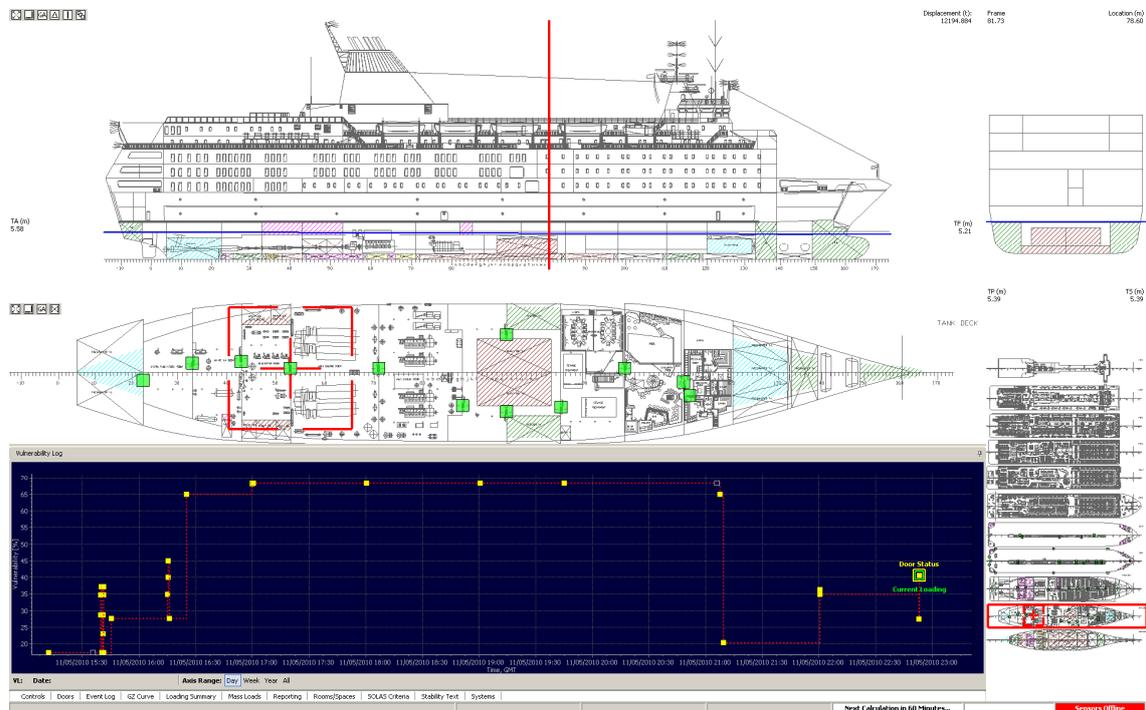
Figure 30 Sample of 8 hours vulnerability log (VLog).
