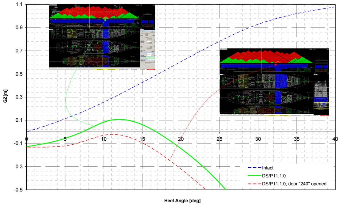
Figure 20 MV Estonia, flooding case No 36, all doors closed, hydrostatic properties.
