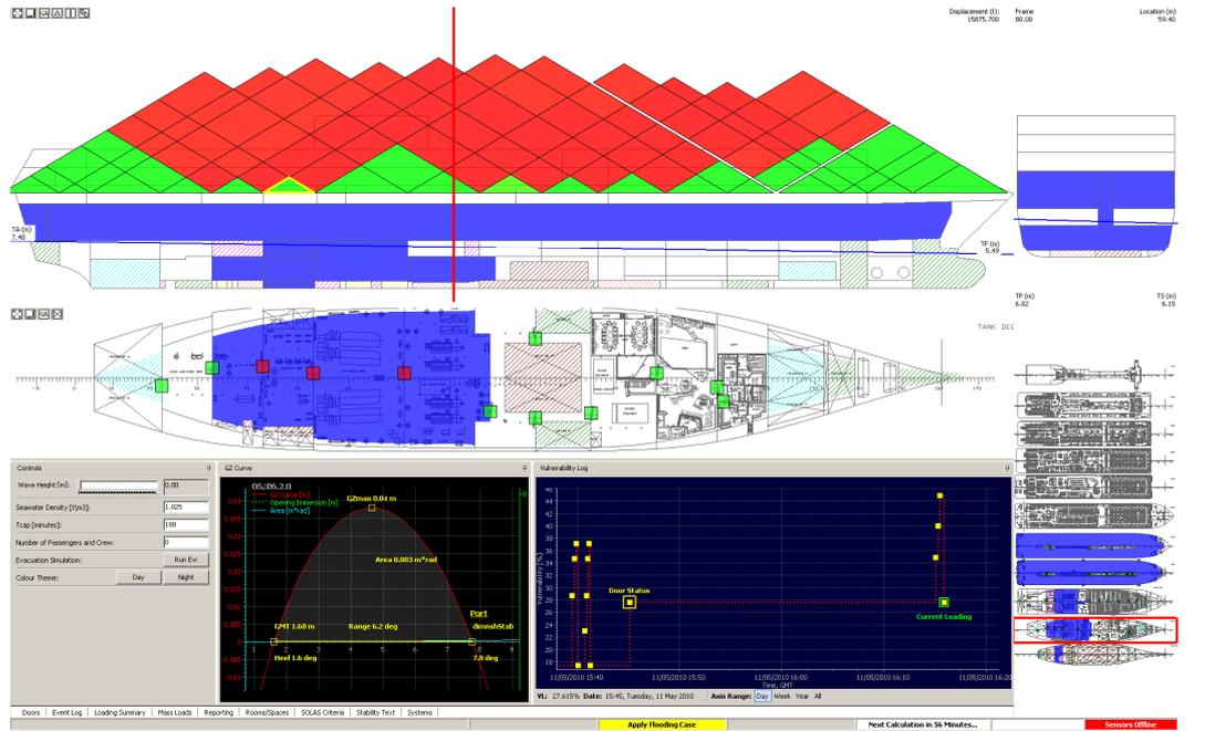
Figure 27 Flooding extent for damage case  $j=702$ , DS/S6.2.0, (diamond/triangle in yellow frame), with corresponding GZ curve logged at 15:45:09, ship vulnerability  $F_T(3hr|0m) = 27.61\%$ . Note the three watertight doors, #216, #217 and #218, on the tank deck opened with the ensuing impact on the flooding extent. Note again  $H_s=0m$ .
