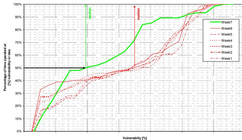
Figure 32 Distribution of vulnerability logged on a demonstration ship. The actual vulnerability values are undisclosed. The impact of the awareness of the crew on the day-to-day management of watertight integrity, and hence crew and ship preparedness, can be seen in the Week 7, when explanation and training on use of VLog had been given.
