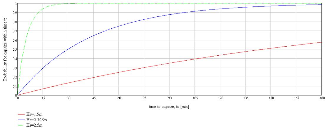
Figure 22 Probability for capsize within time  $t_c$ . Case No 36 with all doors closed. Effect of assumed time to capsize.
