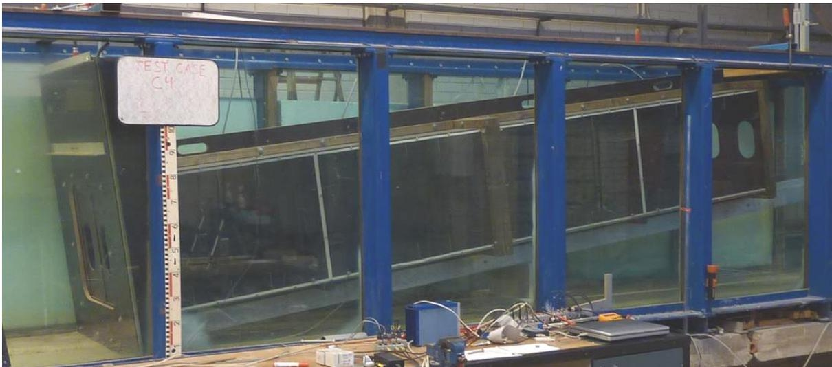
In test case C4 the cross-duct was inclined  $7^\circ$  towards the upstream side. The flow range was very limited due to the flume height. The picture is taken before the test.
