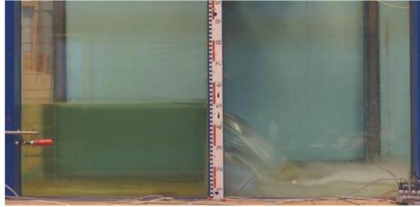
$h_U = 297.2 \text{ mm}$ ,  $Q_A = 152.1 \text{ l/s}$ ,  $Q_T = 252.2 \text{ l/s}$
