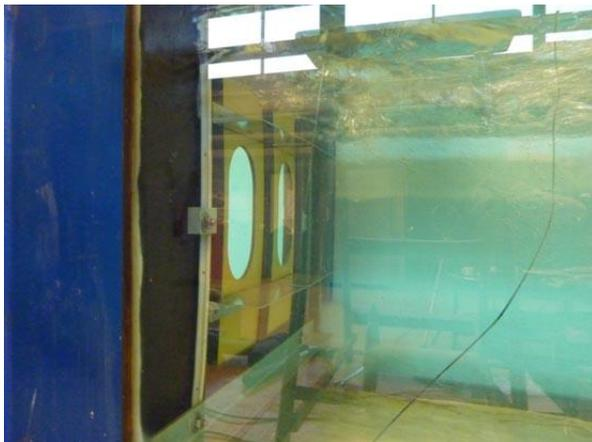
The hydrostatic pressure bends the model girder, which is made of 6 mm thick plywood (test case G3).
