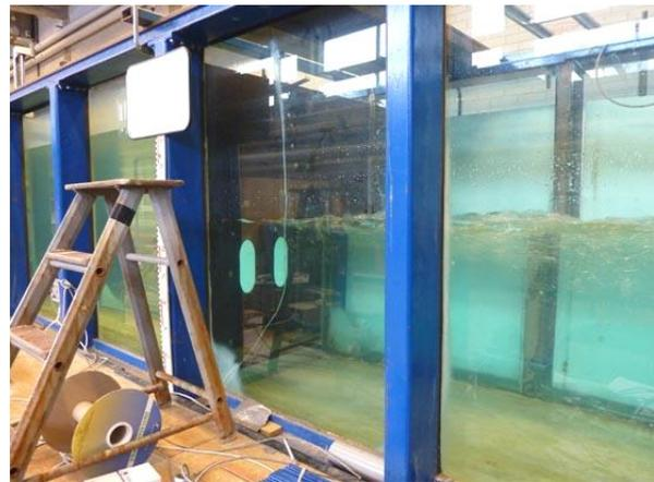
The downstream water surface was quite turbulent with low downstream water levels (G4).
