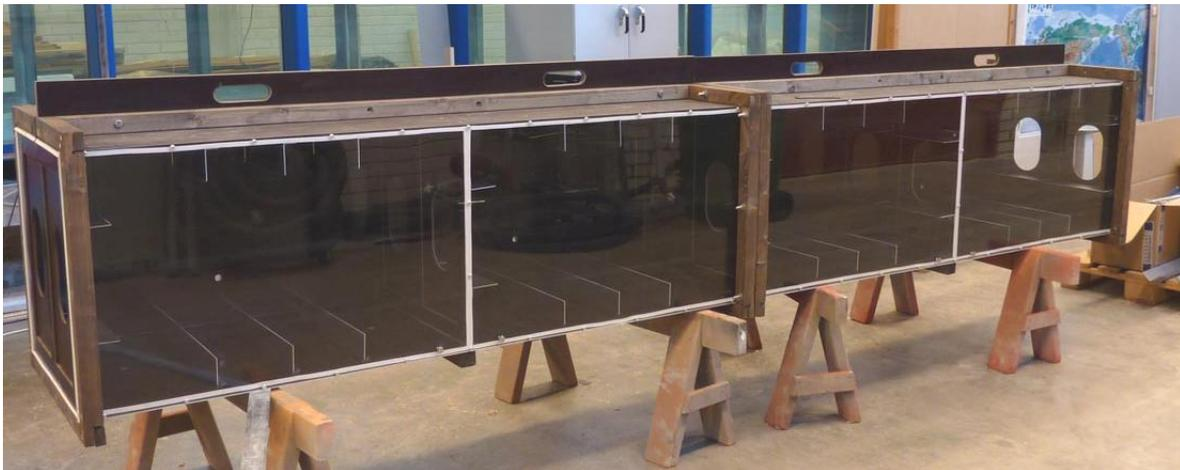
Two cross-duct modules with stiffeners in place and bolted together before test case C2.
