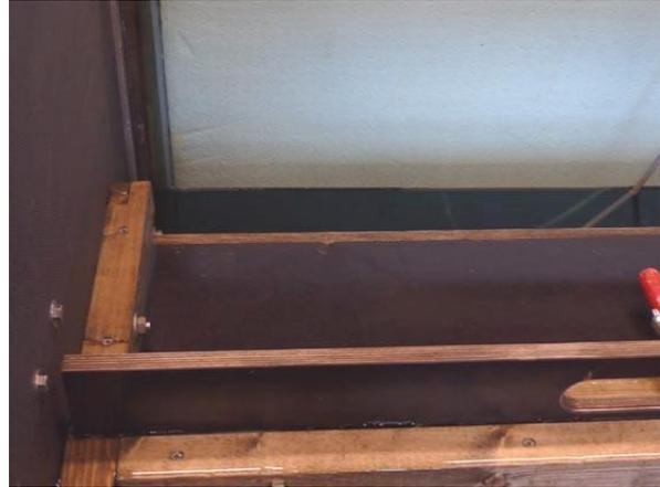
Some leakage was observed between the web-frame plate and the roof of the cross-duct.
