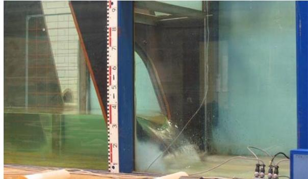
$h_U = 144.5 \text{ mm}$ ,  $Q_A = 25.8 \text{ l/s}$ ,  $Q_T = 45.3 \text{ l/s}$
