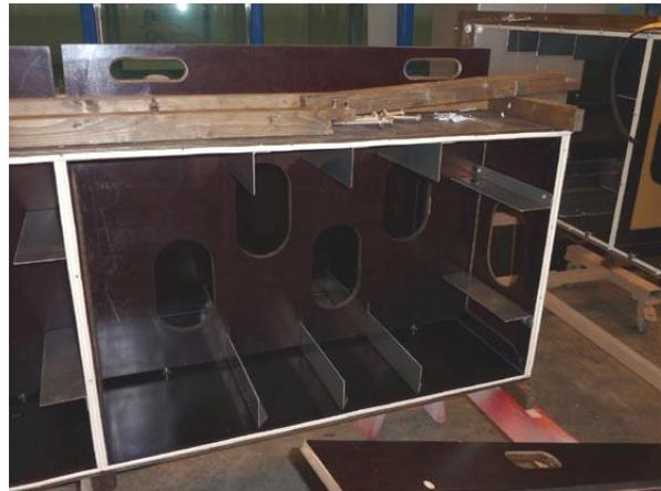
The web-frame plate is fitted in place.
