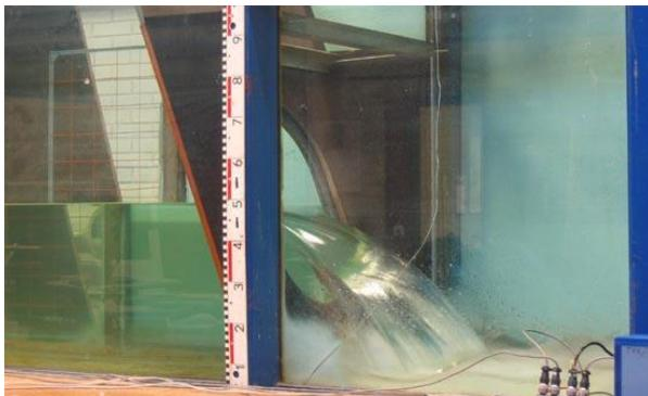
$h_U = 299.2 \text{ mm}$ ,  $Q_A = 93.3 \text{ l/s}$ ,  $Q_T = 168.5 \text{ l/s}$
