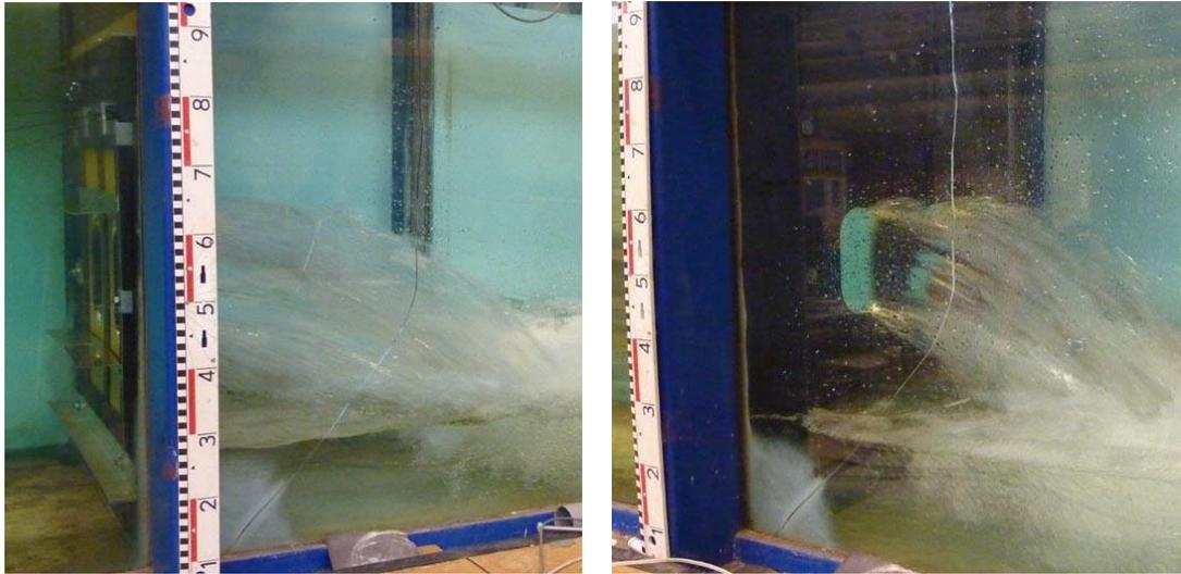
Figure 41. Free flow through a girder with the stiffeners pointing in the upstream direction (test case G4). The jet is smooth on the sides, but incompletely contracted on the bottom and the top.
