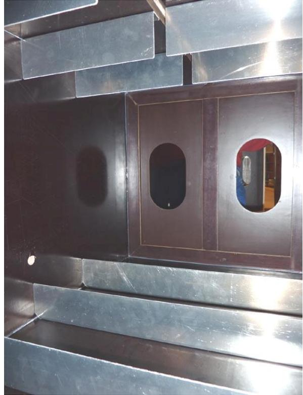
The stiffeners in the compartment roof were made of two parts in order to leave space for the web- frame plate.
