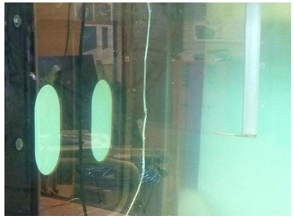
The velocities on the downstream side of the girder was measured with a Prandtl tube.
