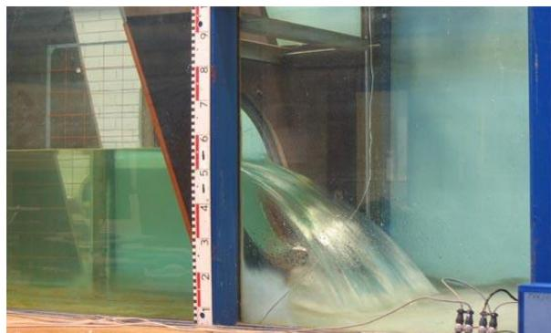
$h_U = 376.8 \text{ mm}$ ,  $Q_A = 138.1 \text{ l/s}$ ,  $Q_T = 249.1 \text{ l/s}$
