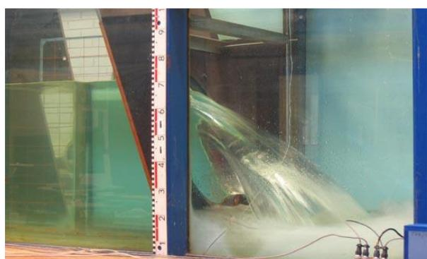
$h_U = 528.2 \text{ mm}$ ,  $Q_A = 238.0 \text{ l/s}$ ,  $Q_T = 428.2 \text{ l/s}$
