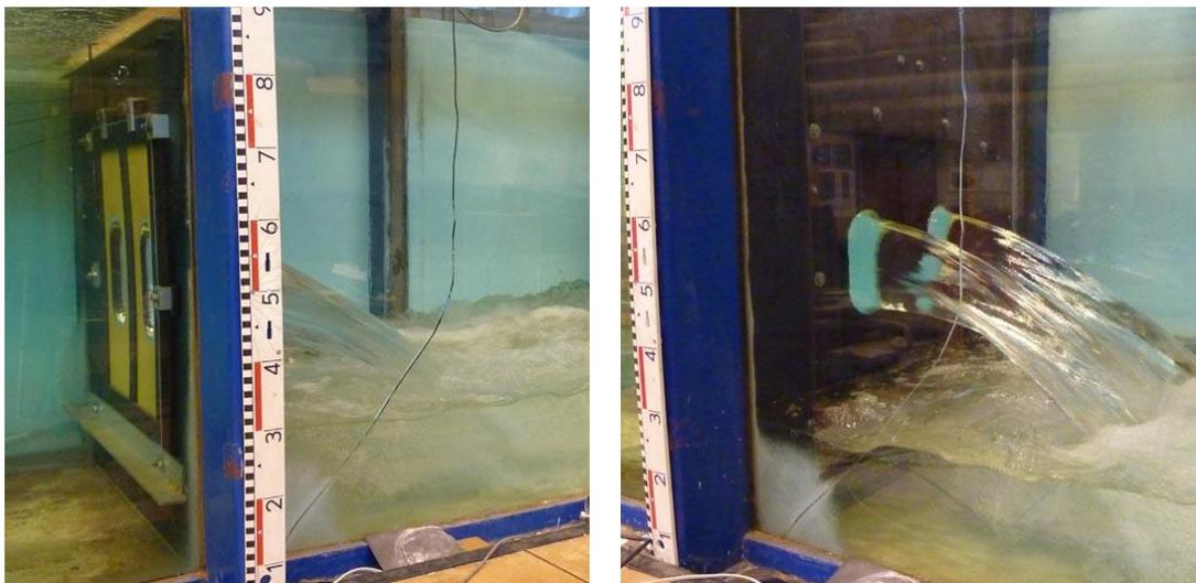
Figure 42. Free flow through a girder without stiffeners (test case G5). The jet is smooth all around. The free flow case with stiffeners pointing downstream is similar.
