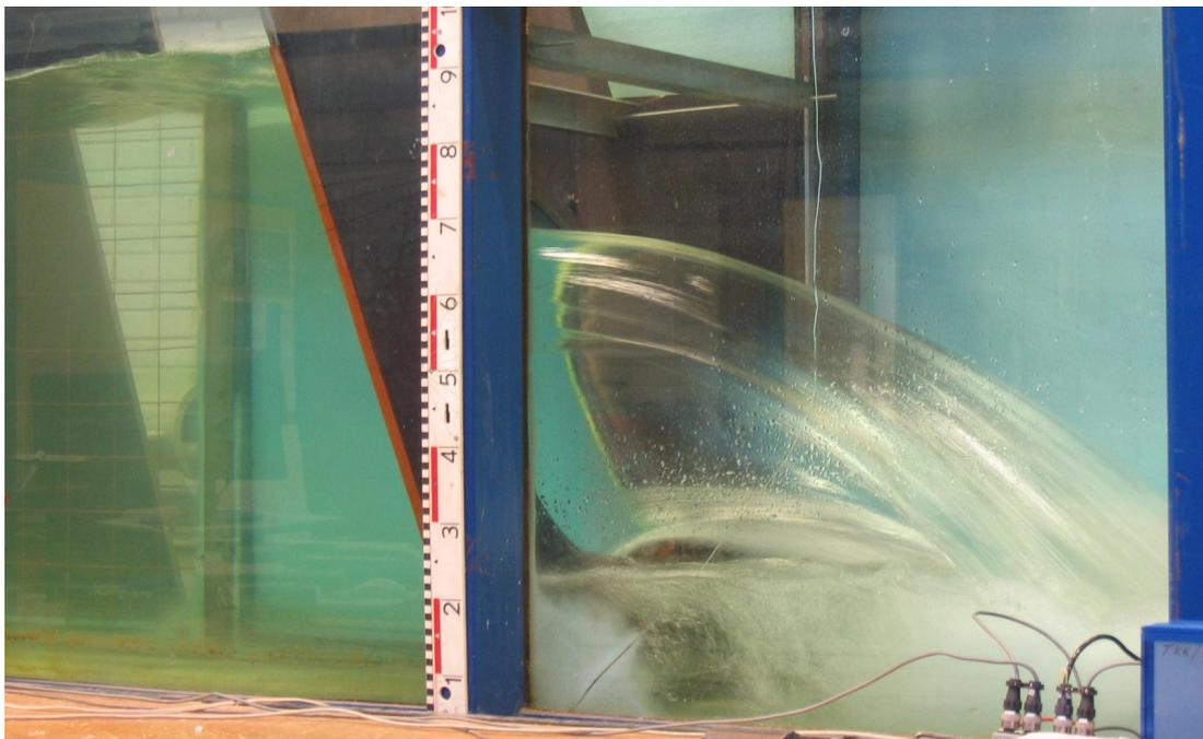
Figure 33. In test case I1 the full-scale manhole was inclined at an angle of 20° towards the flow. Orifice flow is shown with the maximum discharge of  $Q_A = 366$  l/s.
