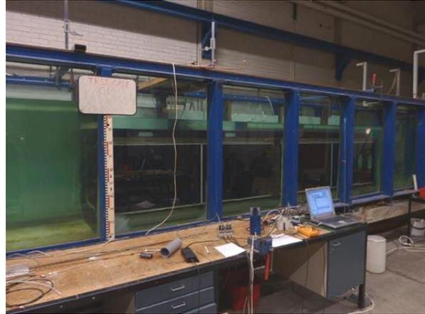
Test case C1. The downstream water level was raised with a tailgate.
