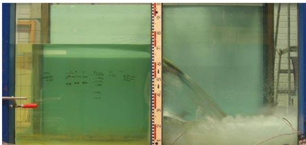
$h_U = 533.5 \text{ mm}$ ,  $Q_A = 237.5 \text{ l/s}$ ,  $Q_T = 408.7 \text{ l/s}$
