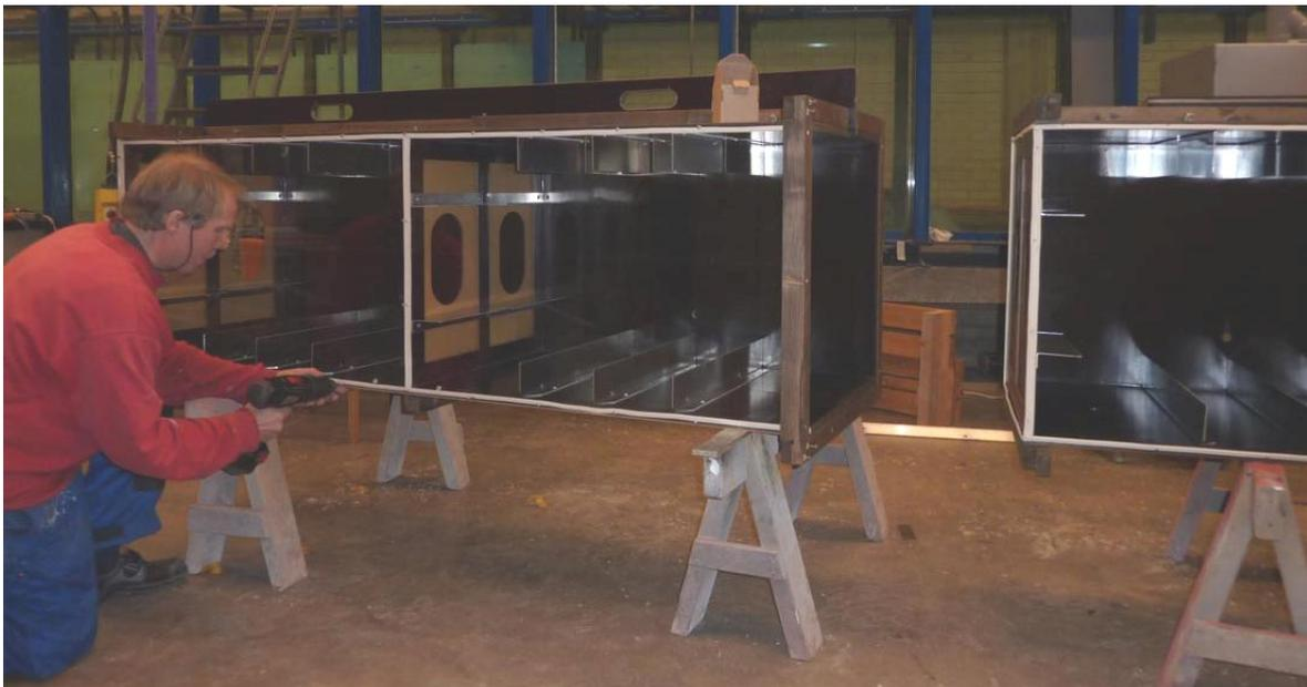
After test case C1, the plexus glass was removed and model stiffeners were added into the compartments and girders. The plexus glass was then fastened again.
