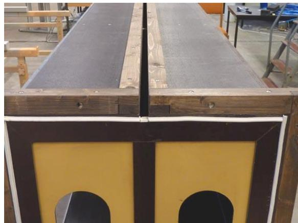
There was an opening on the top of the cross-duct for the web frame plates. The opening was sealed with a plywood plate during the tests.
