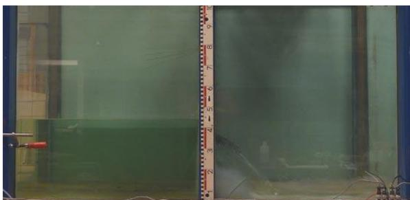
$h_U = 471.5 \text{ mm}$ ,  $Q_A = 282.8 \text{ l/s}$ ,  $Q_T = 463.7 \text{ l/s}$
