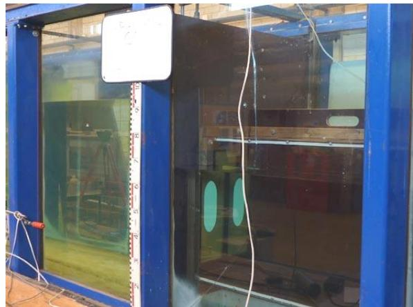
The upstream end of the cross-duct with the dam plate during test case C1.
