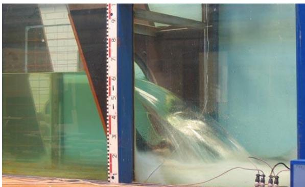
$h_U = 447.5 \text{ mm}$ ,  $Q_A = 183.1 \text{ l/s}$ ,  $Q_T = 331.1 \text{ l/s}$
