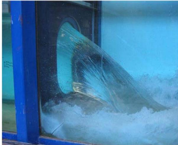
Figure 2 Flow through single manhole (from AALTO)
