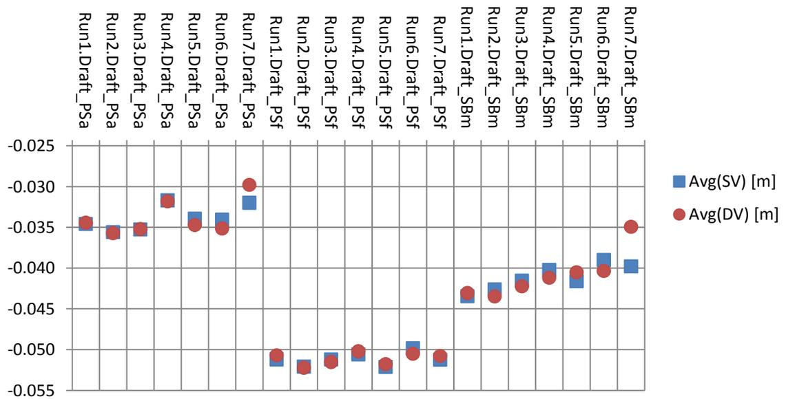
Figure 23 - Measured Drafts (Vacuum)
