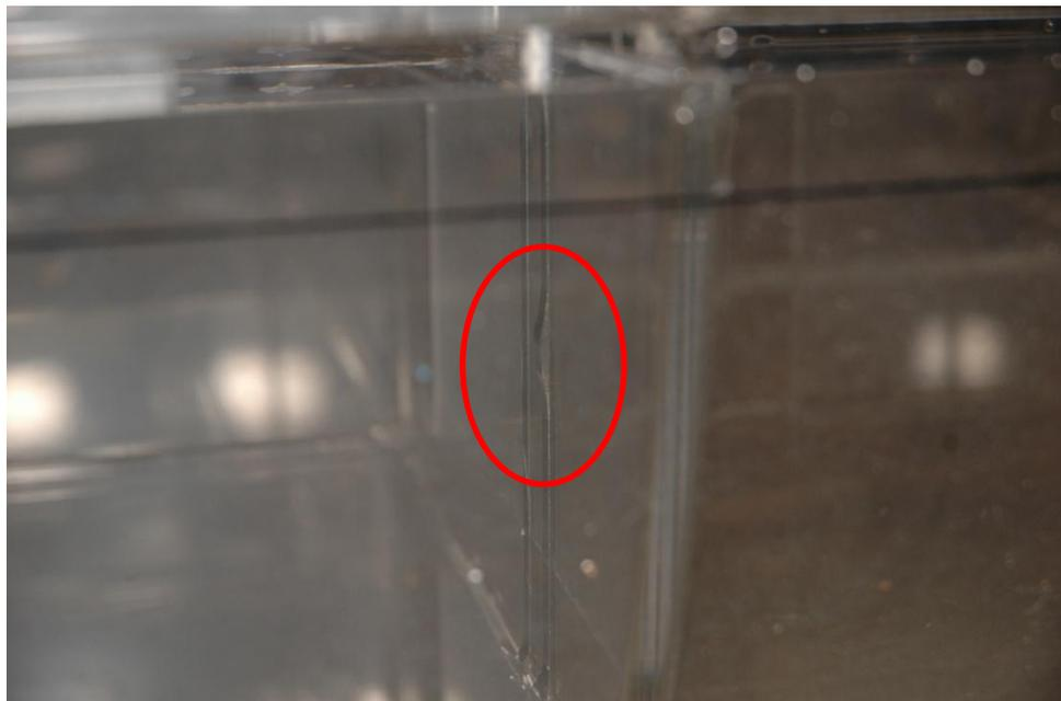
Figure 11 - Detached wave probe
