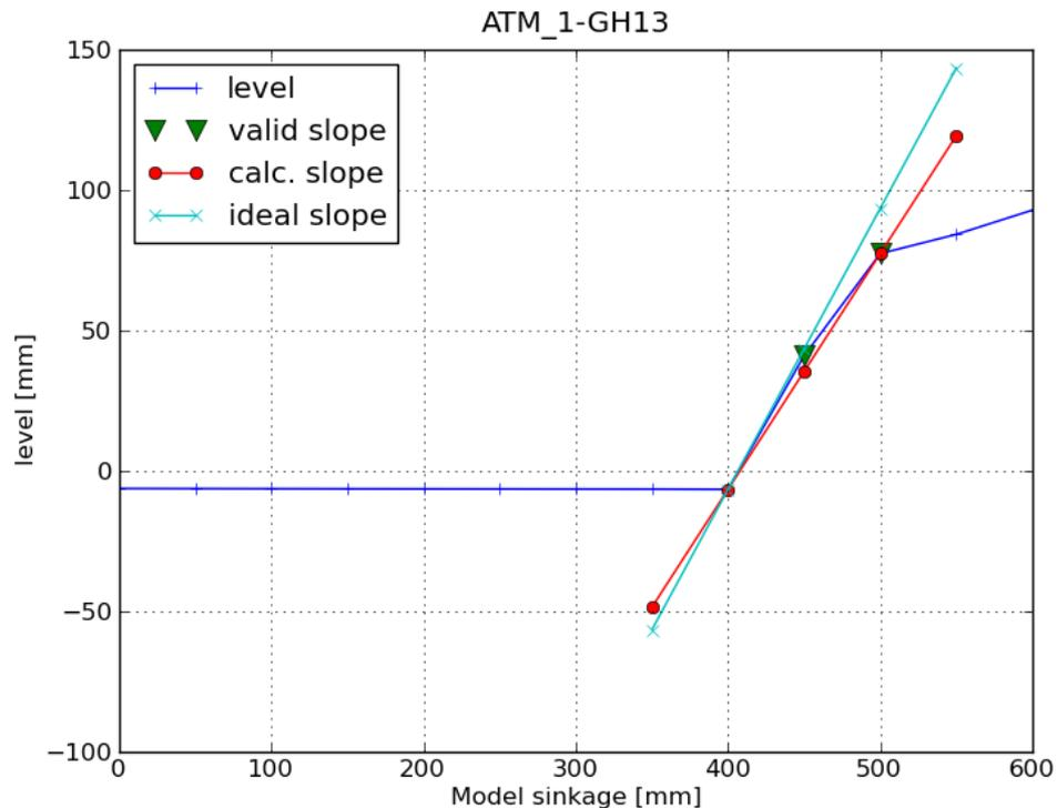
Figure 17 Calibration results (Sensor GH13, simple model, atmospheric)
