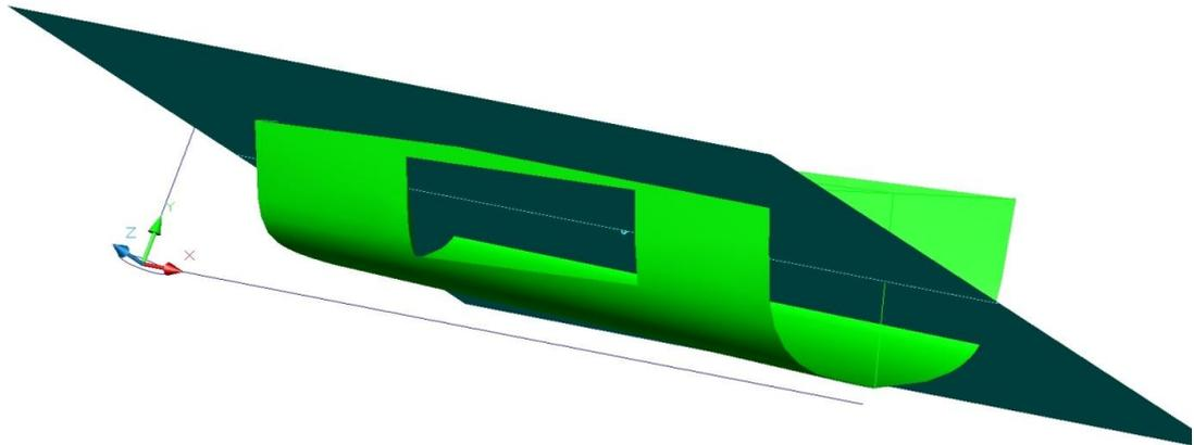
Figure 5 Water plane & Damage opening
