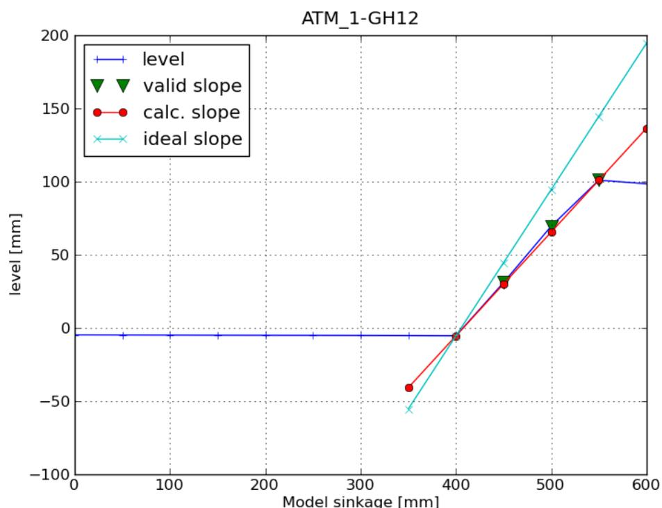
Figure 16 Calibration results (Sensor GH12, simple model, atmospheric)
