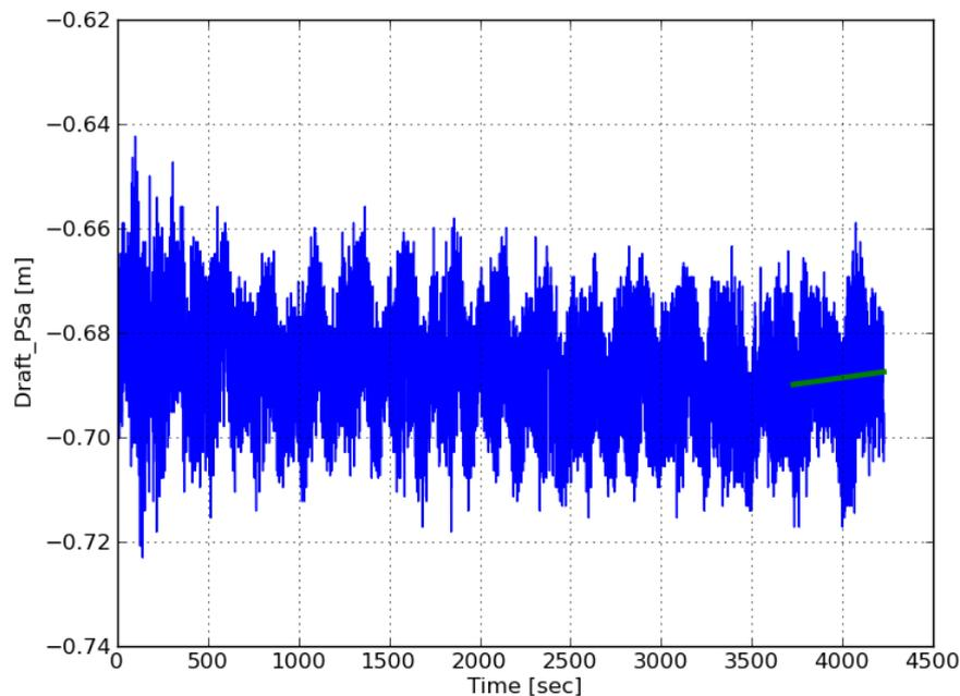
Figure 24 - Draft increase due to flooding (example, full scale)
