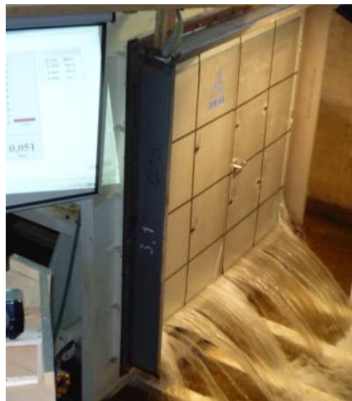
Figure 10: Leakage through A-class double leaf hinged door ( p = 5.1 kPa)
