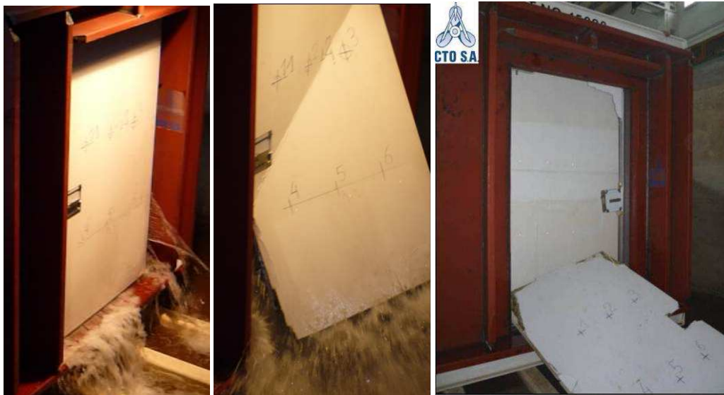
Figure 11: Leakage ( p = 6 kPa) and damage to sliding A-class fire door ( p = 12.8 kPa)
