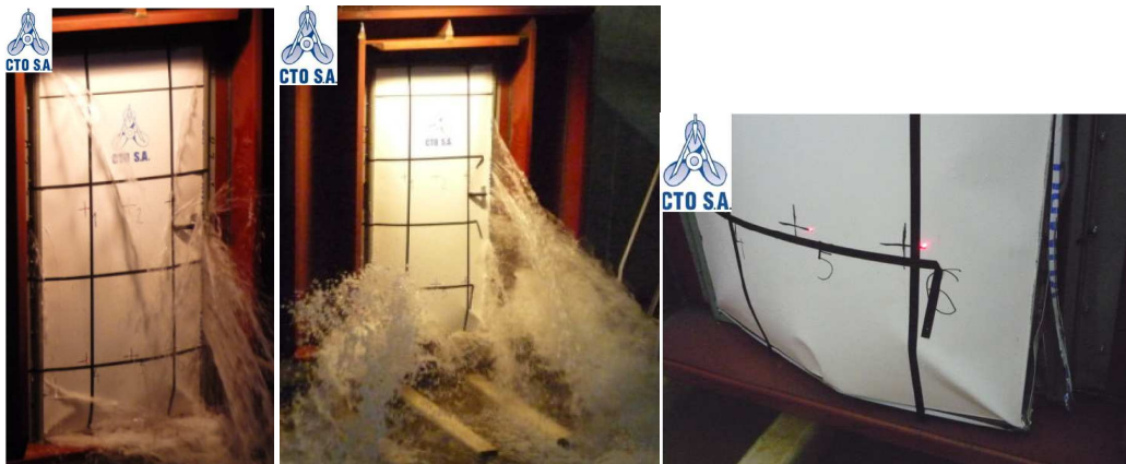
Figure 7: A-class hinged door leaking (left, p = 26 kPa) and damage
