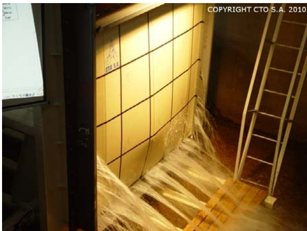
Fig. 2 A non-watertight wall panel leaking in the tests at CTO.
