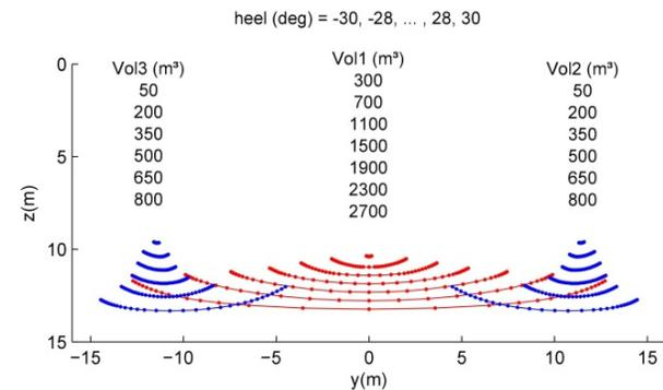
Fig. 2: Location of the lumped mass in compartment 1, 2 and 3 at different flood water volume for heel angles from -30 deg to 30 deg.
