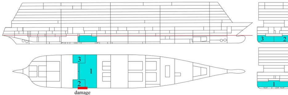
Fig. 1: Flooded compartments.
