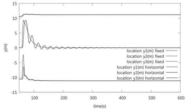
Fig. 5: Flood water transversal location at each compartment.
