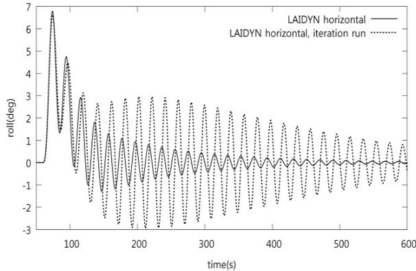
Fig. 7: Forced roll angle at the NAPA simulation and dynamic roll angle.
