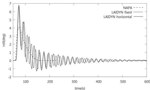
Fig. 3: Heel and roll angle at the quasi-static and dynamic simulation.
